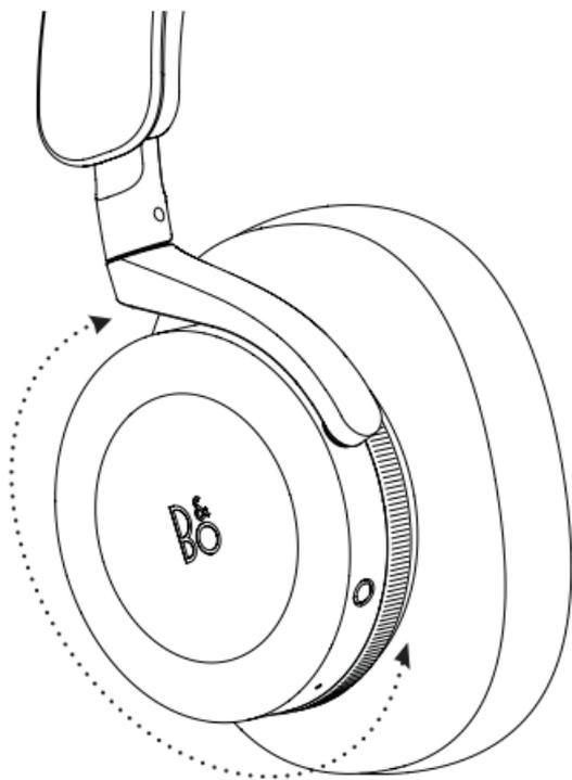
Rotate the dial on the left ear cup to adjust between Active Noise Cancellation and Transparency Mode.
