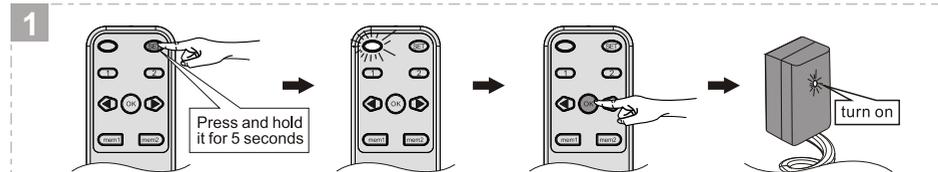
Press and hold the "SET" button for 5s. When the LED indicator on the remote control lightens continuously, press the "OK" button. The buzzer will beep once. After the IR receiver lightens, the system enters learning mode.
