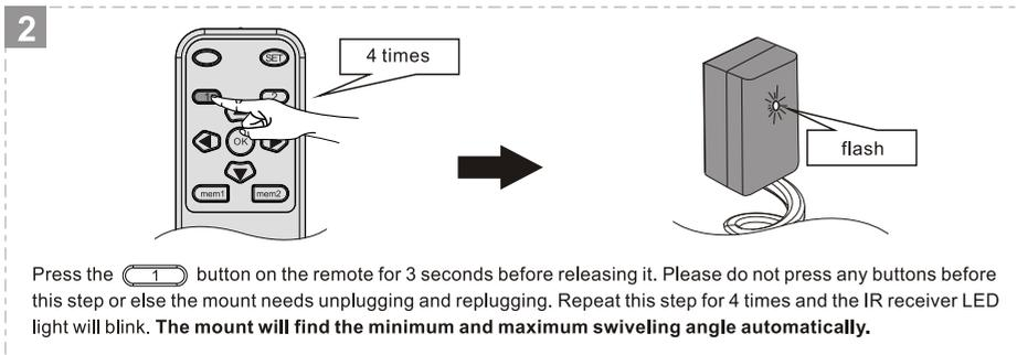
Press the **1** button on the remote for 3 seconds before releasing it. Please do not press any buttons before this step or else the mount needs unplugging and replugging. Repeat this step for 4 times and the IR receiver LED light will blink. **The mount will find the minimum and maximum swiveling angle automatically.**
