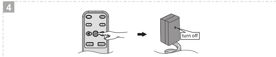
Press the "OK" button. The buzzer will beeps 4 times, and the IR receiver turn off. The duplication is successful.
