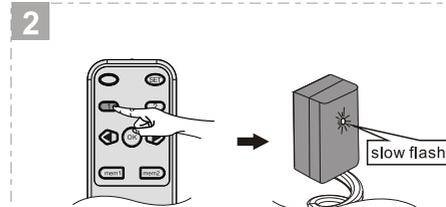
Long press the "1" button for 3s. The buzzer will beep twice, and the IR receiver will flash slowly.
