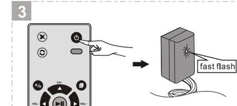
Target your TV remote control at the IR receiver, and press a button that is correspondent with the function of "Power" button. Then, the buzzer beeps three times, and the IR receiver flashes quickly.
