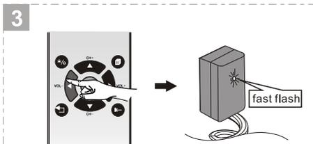
Target your TV remote control at the IR receiver, and press a button that is correspondent with the function of "Power" button. Then, the buzzer beeps three times, and the IR receiver flashes quickly.
