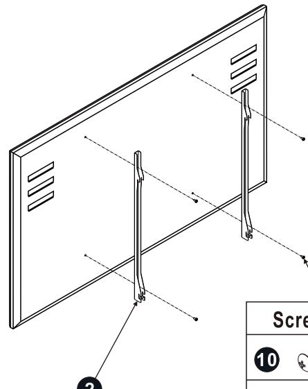
V. Once Stand is assembled, Pre Adjust the springs according to the weight of the TV or Monitor as per the adjustment chart. (Page 4). An even number of turns for each side will facilitate weight balance and easy final adjustment.
