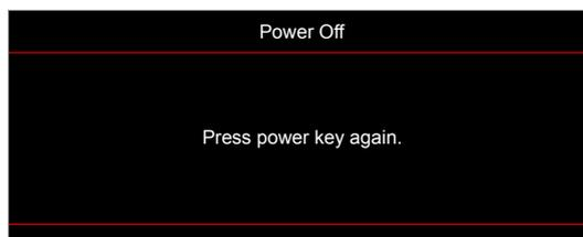
3. Press the  $\cup$  or | button again to confirm, otherwise the message will disappear after 15 seconds. When you press the  $\cup$  or | button for the second time, the projector will shut down.
