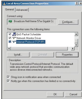
6. Type in the IP address and Subnet mask, then press “OK”.
