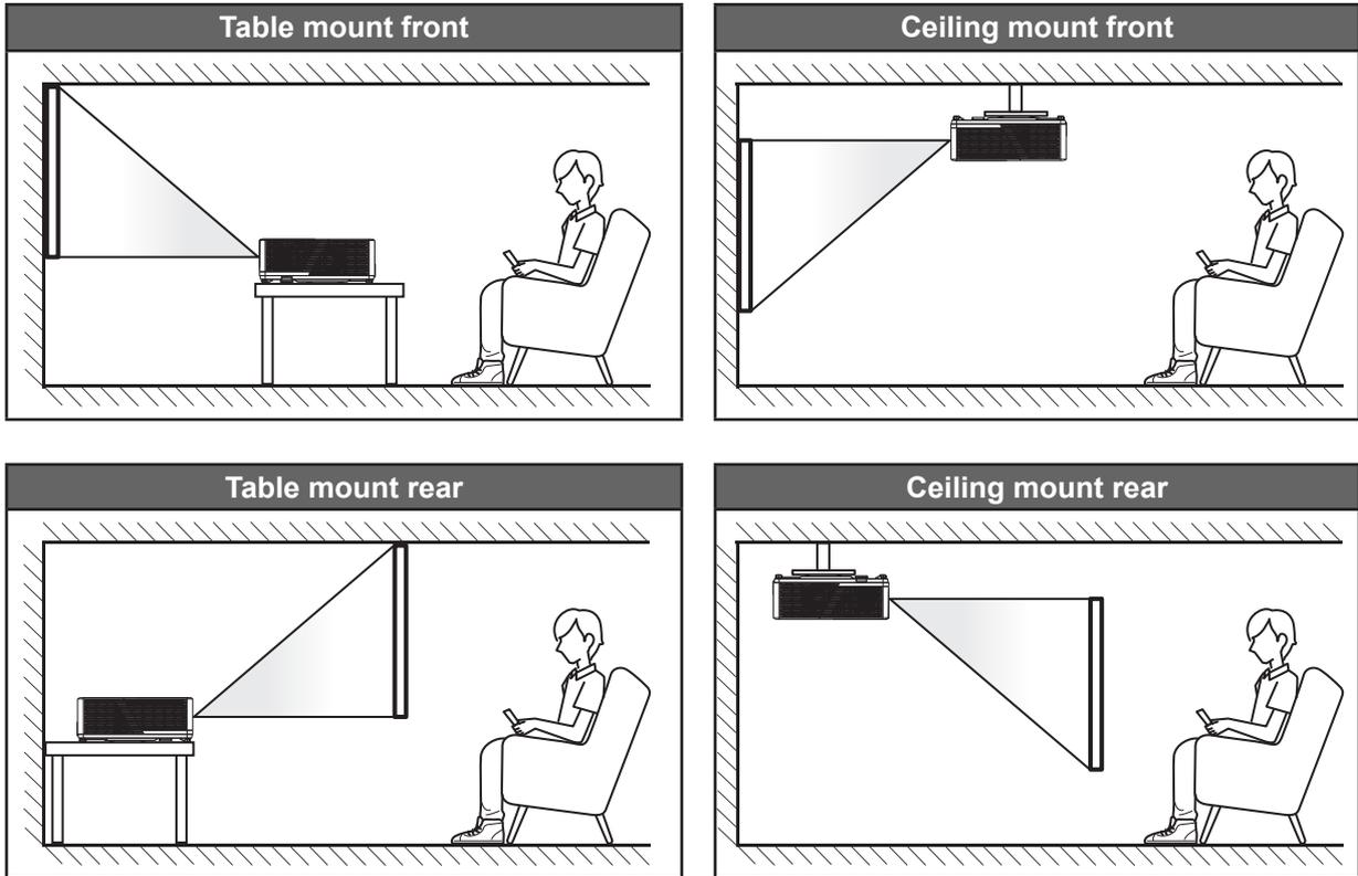
Projector should be placed flat on a surface and 90 degrees / perpendicular to the screen.
