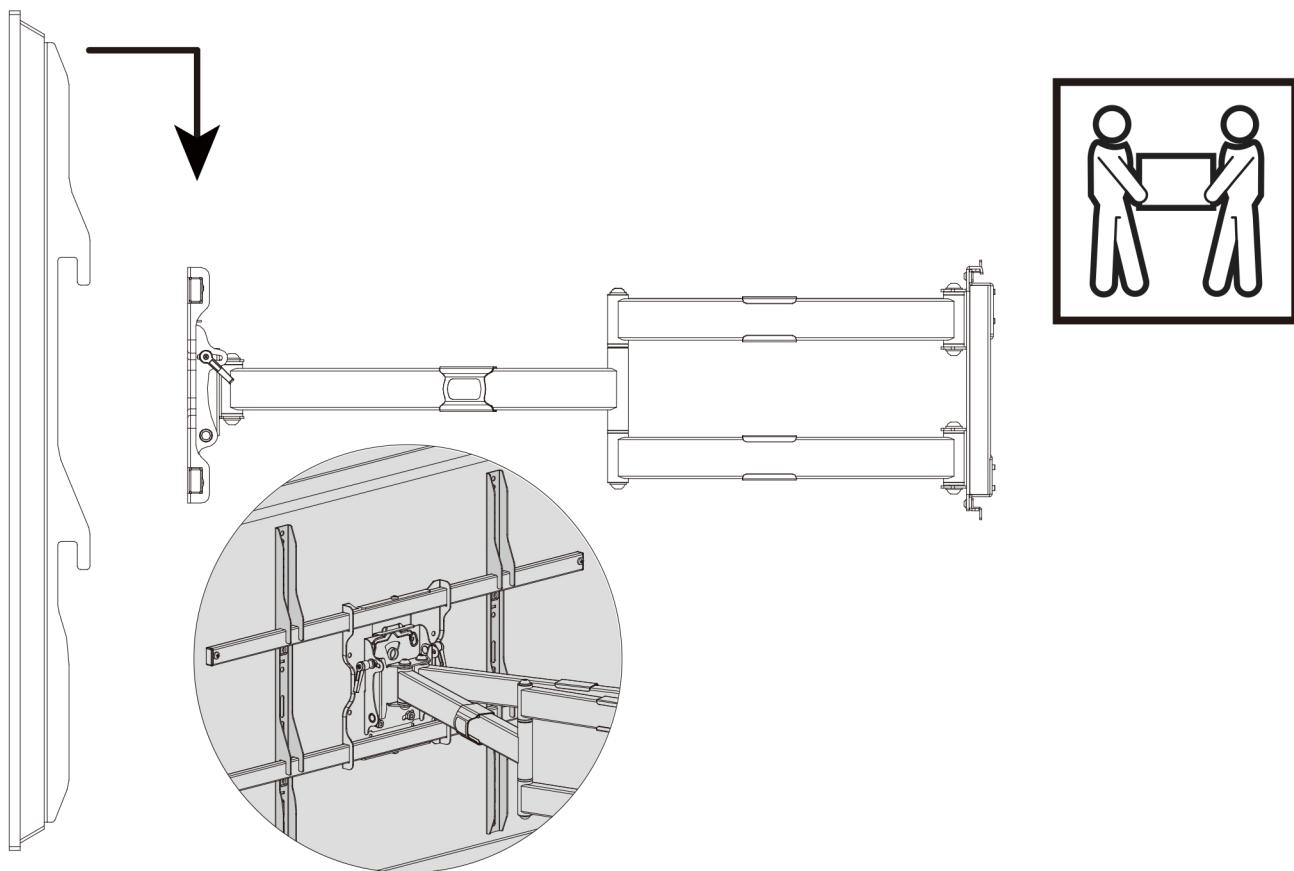
Lift the TV up (two persons recommended) and hang the TV brackets on to the wall mount extension bars.
