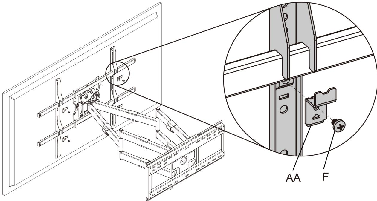
Secure the TV brackets on the mount by attaching the 4 x AA Safety Brackets with 4 x F Screws as shown on the image.
