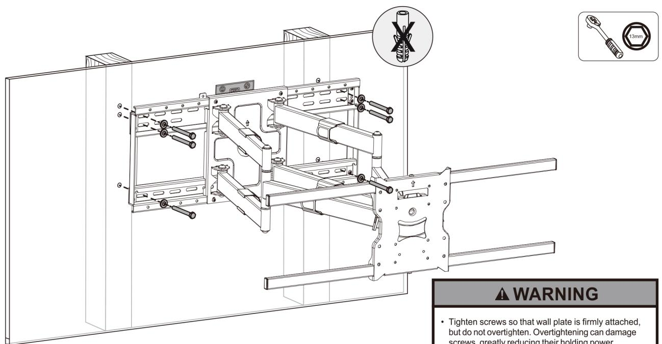
Secure the Wall Plate to the wall with 6 x Lag Bolts ( H ) and 6 x Washers ( H ). NOTE: Do not use Wall Anchor ( I ) for wood stud installation.
