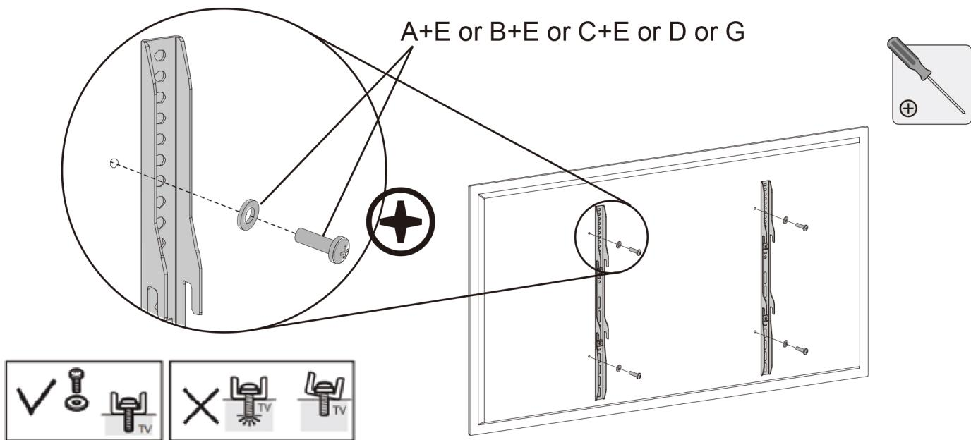
Attach the 2 x TV Brackets to the back of the TV by using screws A+E or B+E or C+E or D or G.
